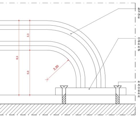
20 DETALHE BARRA DE APOIO PCD
